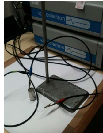
Figure 1: Miniaturised ILW drum system being corroded in the lab.
