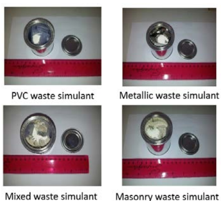
Fig1: (Left) Laboratory scale PCM mock up drums, with addition of 1.04 wt% \text{CeO}_2 , as a Pu surrogate. (Center) Addition of glass forming frit at a 1:1wt% ratio with waste simulants. Thermal treatment 1560^\circ\text{C} Melting temperature for 4 hours. (Right) example of vitrified waste product, masonry in this case.
